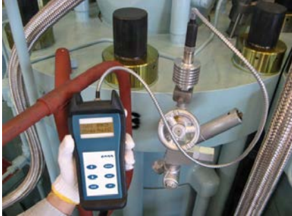
Fig. 3. EPM-XP application on MAN B&W two-stroke diesel engine built under license by Kawasaki Heavy Industries (IMES GmbH 2018d)
